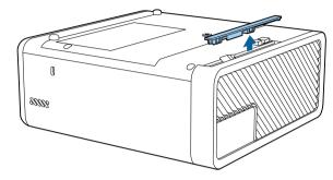
Pull the air filter out of the projector.
