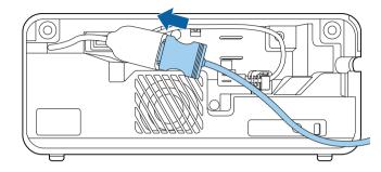
Pass the HDMI cable through the cable path as shown.
