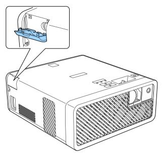
Connect the stereo headphone's mini-jack cable to the projector's Audio Out port.
