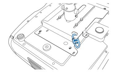
Attach the wire clamp to another carabiner, and then use the screw to fix the wire clamp to the wire clamp fixing point on the projector.
