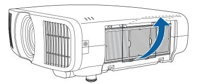
Pull the air filter out of the projector. 5
