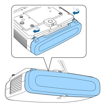
To remove the cover, loosen the cover screws and pull the cover off of the projector.
