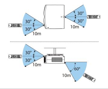
• Avoid using the remote control in conditions with bright fluorescent lights or in direct sunlight, or the projector may not respond to commands. If you are not going to use the remote control for a long time, remove the batteries.
