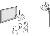
Select the correct **Projection** option in the projector's **Installation** menu according to the installation method being used. If necessary, turn on the **Inv Direction Button** setting in the projector's **Operation** menu.
